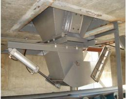
Tunnel Gate made of A.R. steel
