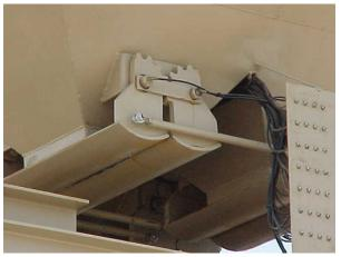
Agg Bin gate with grease fitting panel
