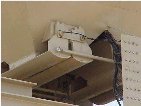
Agg Bin gate with grease fitting panel
