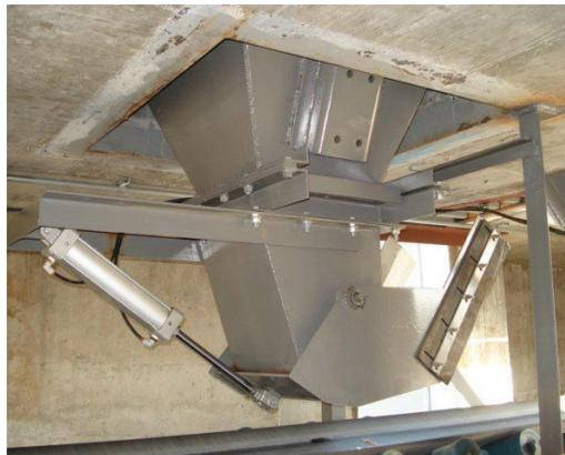
Tunnel Gate made of A.R. steel
